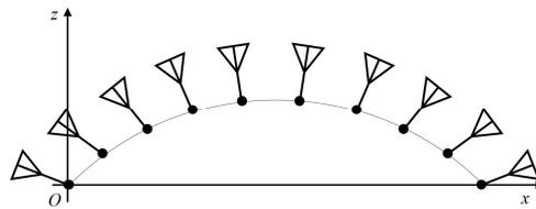
Fig. 2. Ten-element misaligned antenna array deployed on a globular-shaped surface.
