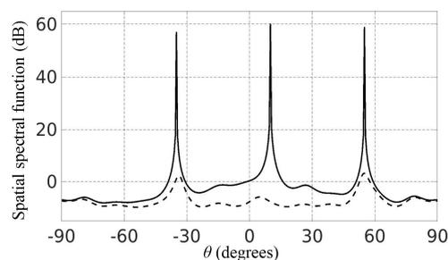
Fig. 3. Comparison between the spatial spectral functions obtained by using the proposed method and the conventional spatial smoothing technique.
