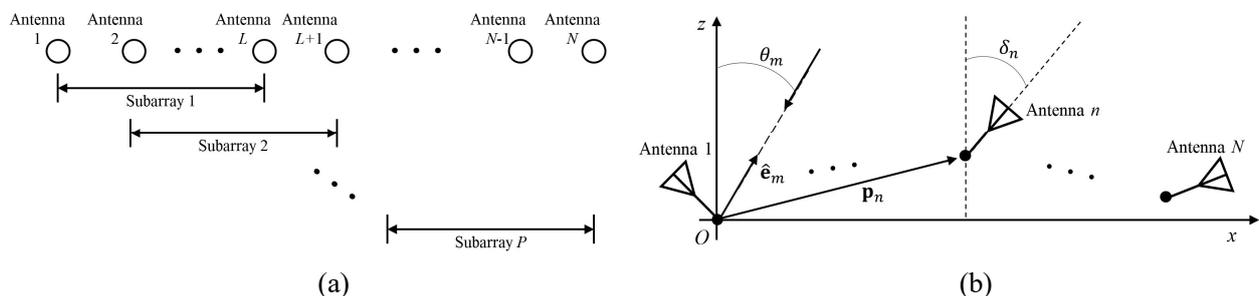
Fig. 1. (a)  $N$ -element antenna array divided total  $P$  subarrays of size  $L$  for spatial smoothing, (b) Coordinate systems for the  $N$ -element misaligned antenna array.
